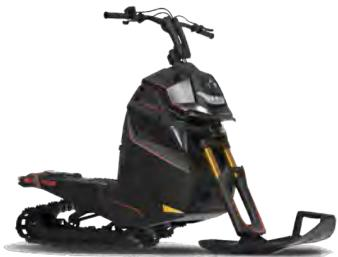
Riders typically stand atop the tunnel on non-slip material, and control the vehicle using traditional throttle and brake controls mounted on a raised handlebar. With its aluminum frame, tunnel and handlebar plus composite bodywork, the WS250
